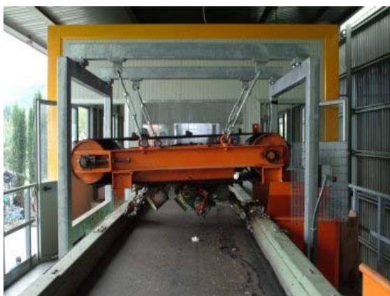
Figura 5.2-12: Separator magnetic automat feroase
